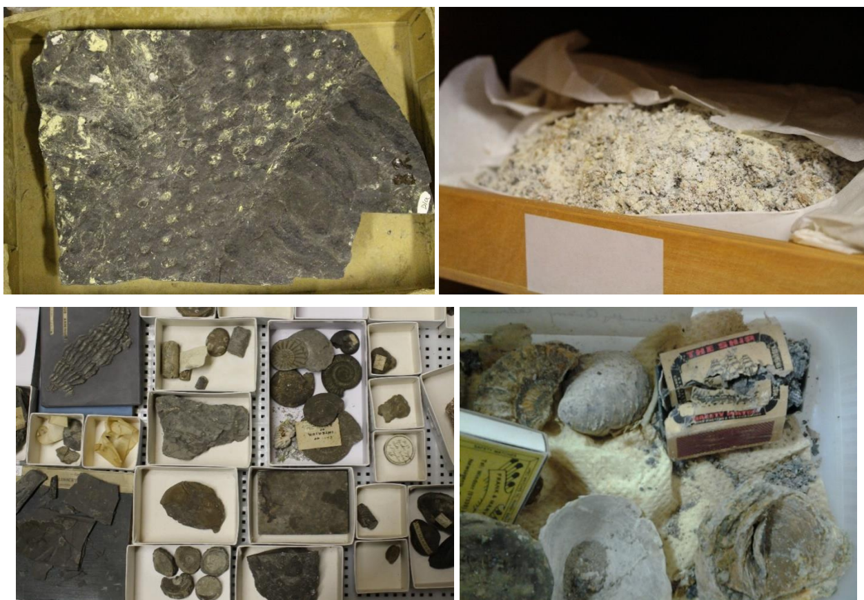
Figure 70: Carboniferous Stigmaria in sulphur-rich coal showing surface discolouration (top left); a fossil reduced to powder by pyrite decay (top right); a drawer with a decayed ammonite (bottom left); and a matchbox damaged by a decayed pyrite fossil (bottom right)
