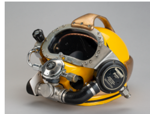
Kirby Morgan diving helmet with Helinaut 350 Gas Reclaim valve. © Aberdeen City Council (Archives, Gallery & Museums Collection).
